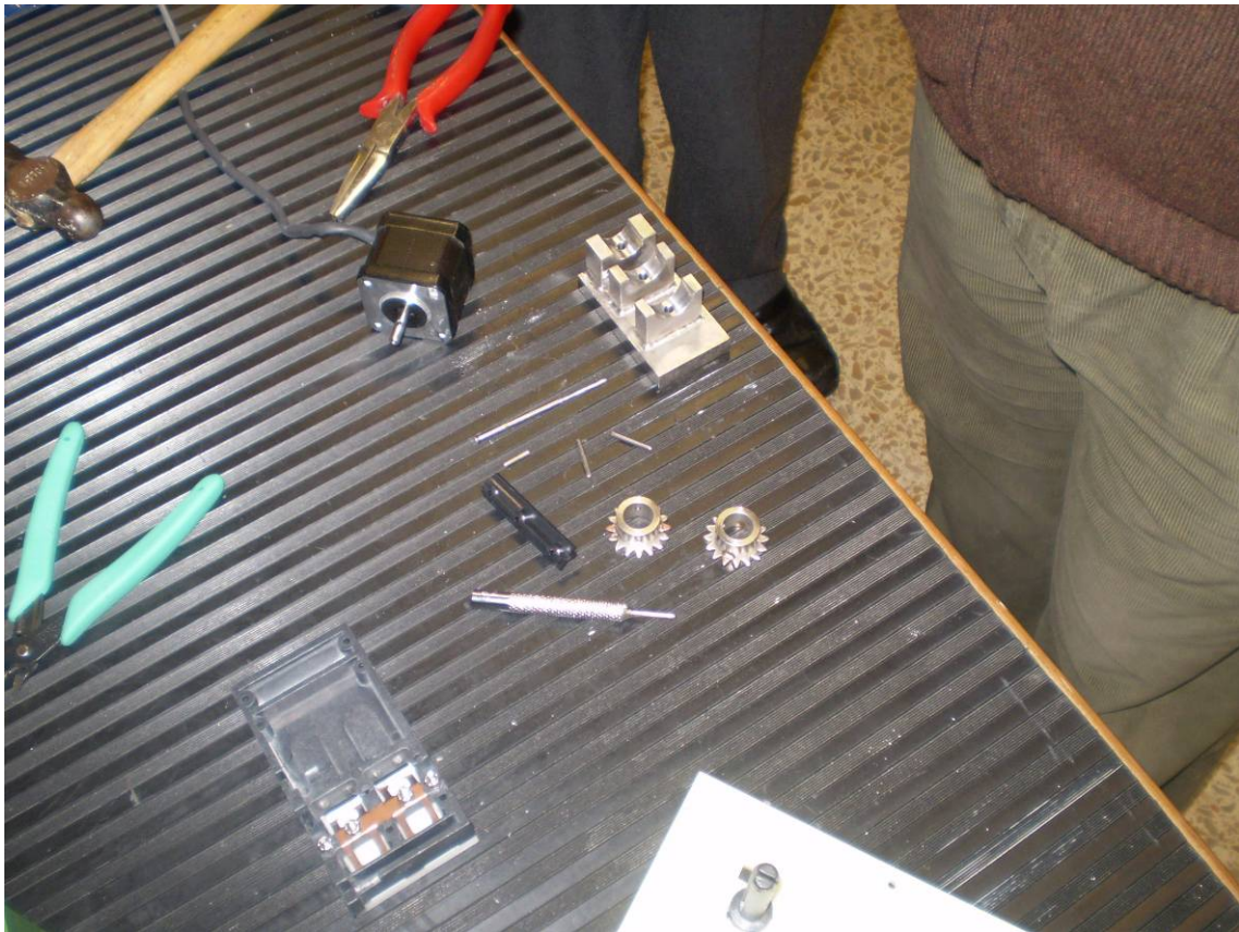
15.- Insert the sprockets on the new shafts and align with the holes
