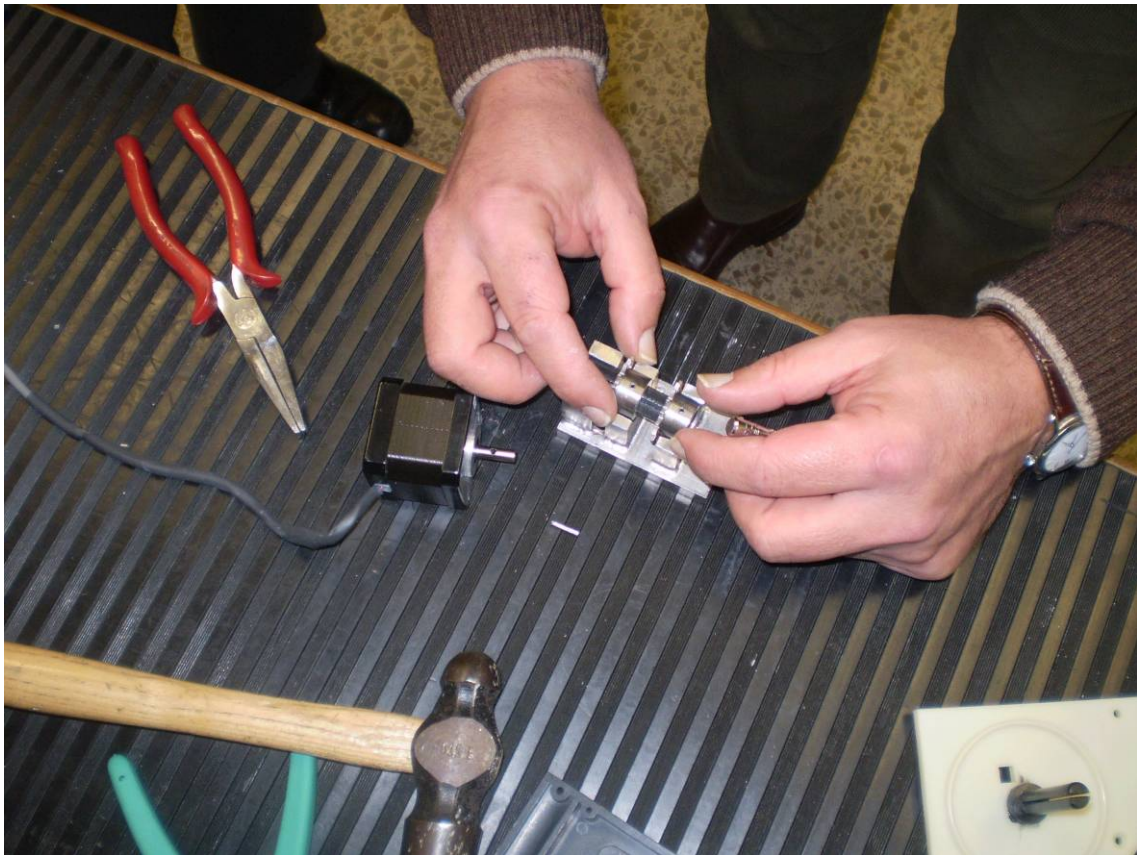
14.- Take out the pins that hold the sprockets in place
