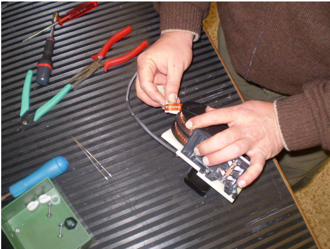
28.- Holding both reels at the same time put both copper tapes on the sprocket and take them out till the contacts
