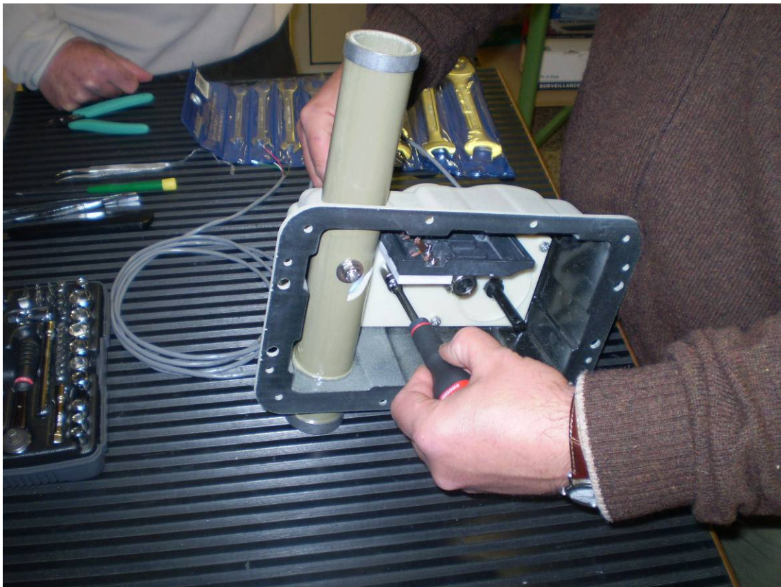
8.- Unscrew the 3 screws that hold the motor plate
