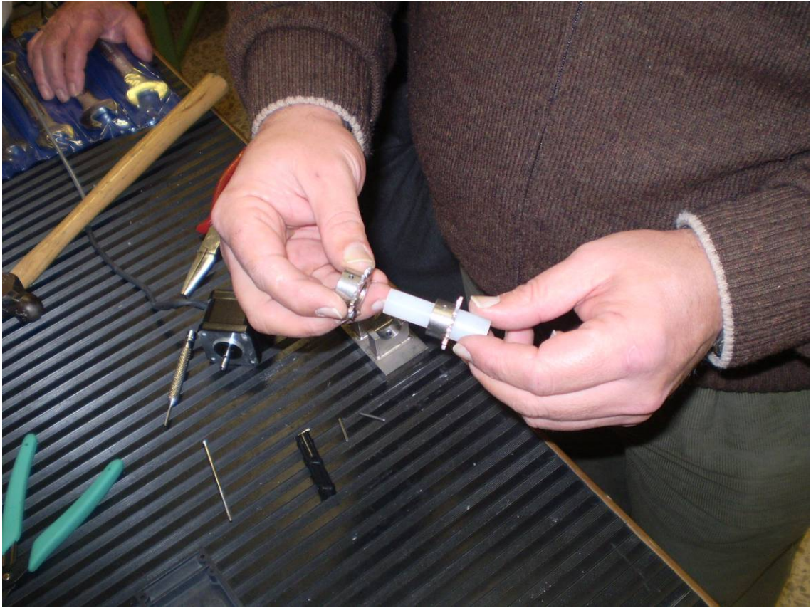
16.- Reinsert the pins on the sprockets using the originals pins
