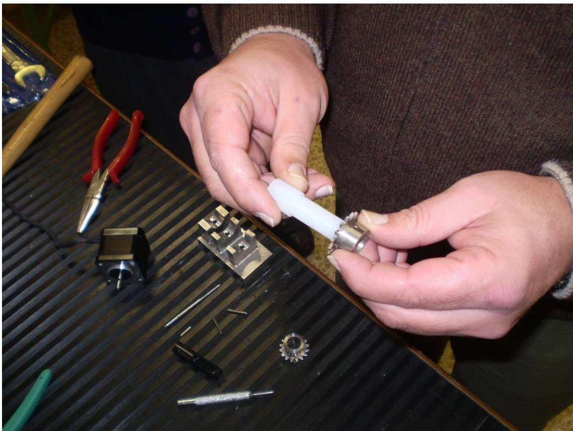
15.- Insert the sprockets on the new shafts and align with the holes
