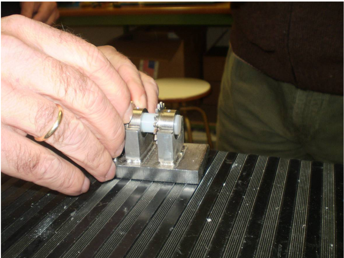
16.- Reinsert the pins on the sprockets using the originals pins
