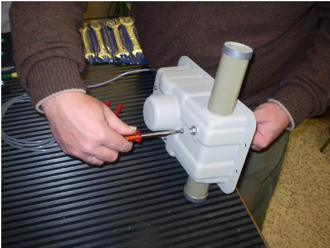
8.- Unscrew the 3 screws that hold the motor plate
